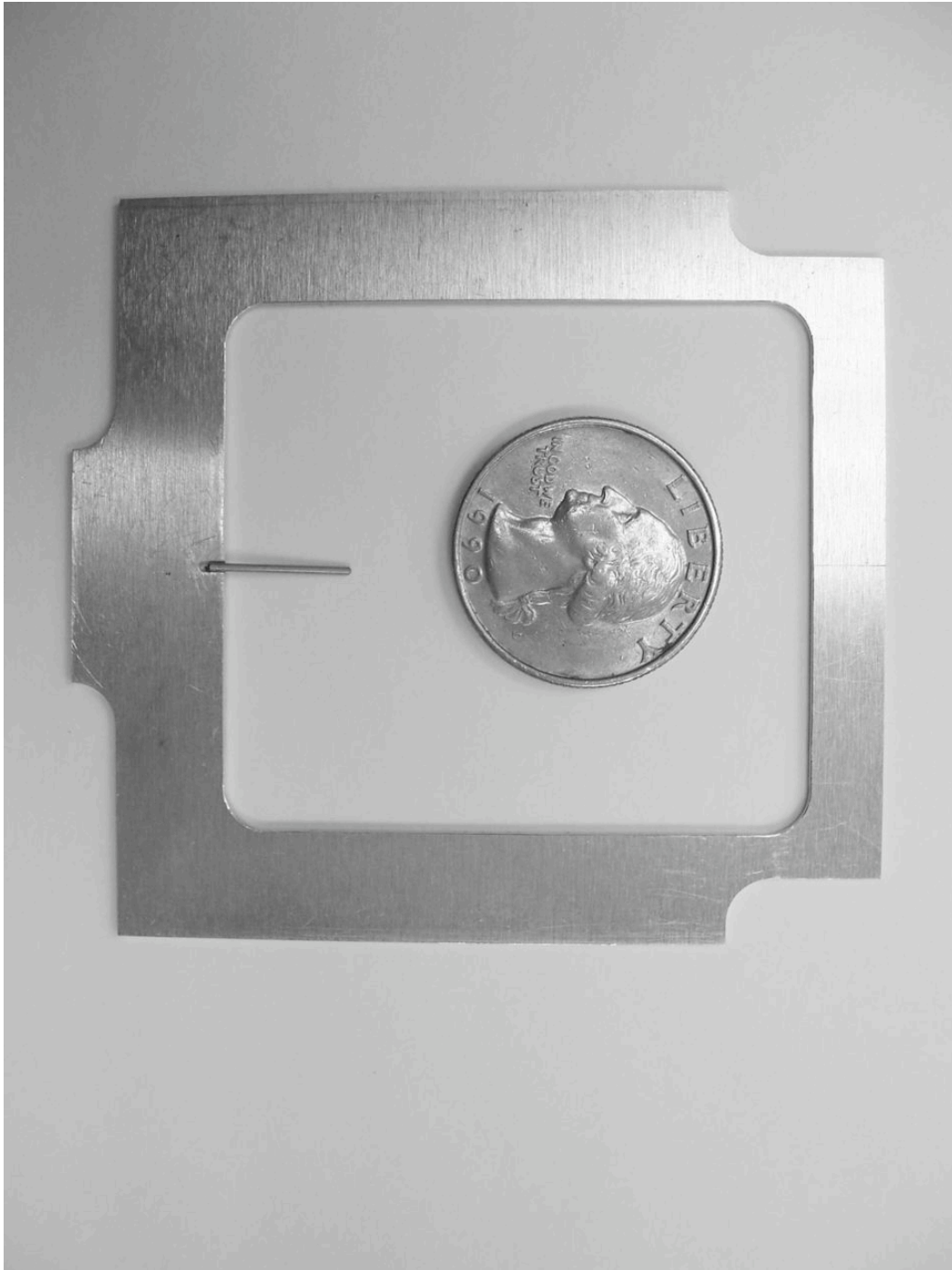
Fig. 13. An image of the alpha calibration source frame and source pin.
